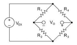
The Wheatstone bridge is the electrical equivalent of two parallel voltage divider circuits.  $R_1$  and  $R_2$  compose one voltage divider circuit, and  $R_4$  and  $R_3$  compose the second voltage divider circuit. The output of a Wheatstone bridge, Vo, is measured between the middle nodes of the two voltage dividers.
