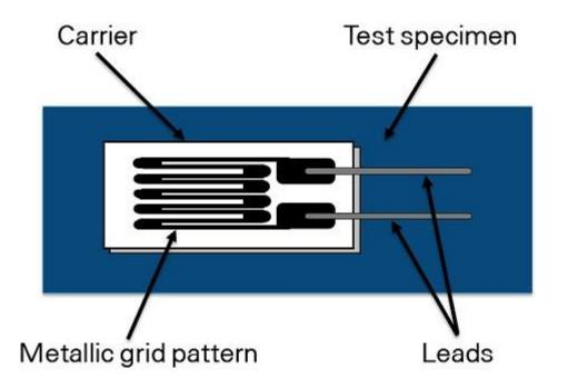
A fundamental parameter of the strain gage is its sensitivity to strain, expressed quantitatively as the gage factor (GF). GF is the ratio of the fractional change in electrical resistance to the fractional change in length, or strain:
