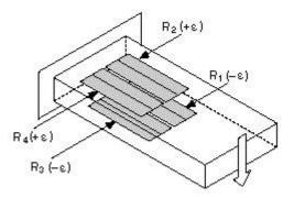
Configuration Type III: Only Axial Strain
