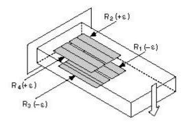
Configuration Type I: Only Bending Strain
